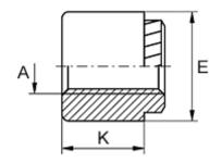
Female thread A= M3Height K= 7Hole diameter +0.1= 4.2Min distance to edge= 2.4Min material thickness= 1.5Outer diameter E= 7
